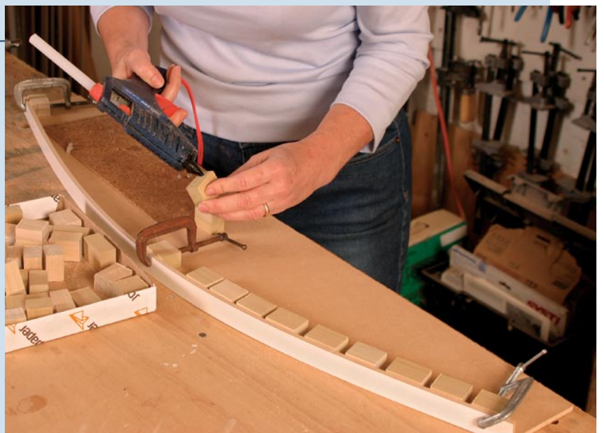
Use more blocks to stiffen the template. Glue more blocks to the base and the back of the strip. Take care not to alter the curve.
