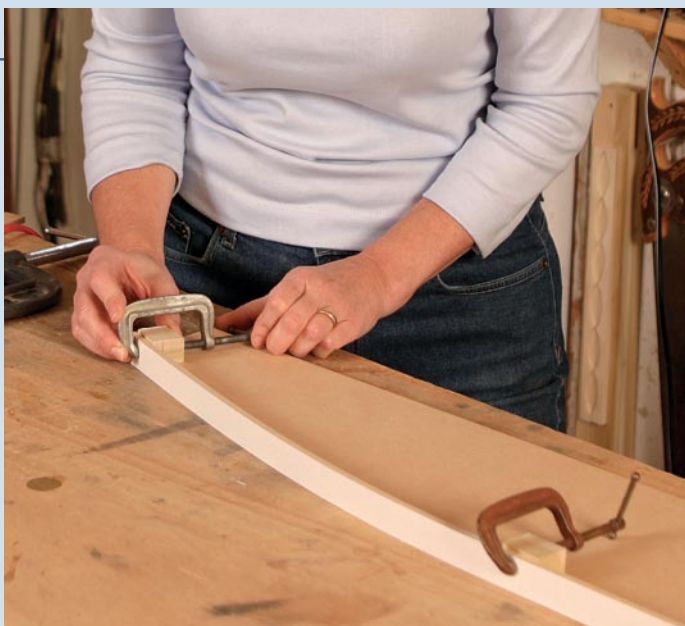
Form the curve. Clamp an edge strip to the three blocks to form a smooth curve.
